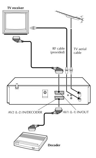
The AV2 (L-2) IN/DECODER connector can be used as an input connector for an external decoder (descrambler). Simply connect a decoder and you can enjoy the variety of programming that is available through scrambled channels.
